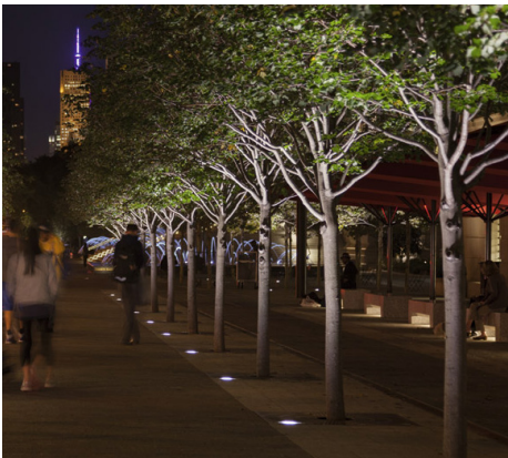
New pedestrian lighting to provide a human scale along the street and improve safety in the area. Provide a combination of in-ground lighting to enhance trees with linear lighting projected on the ground from under side of benches and key locations such as brick heritage wall.
