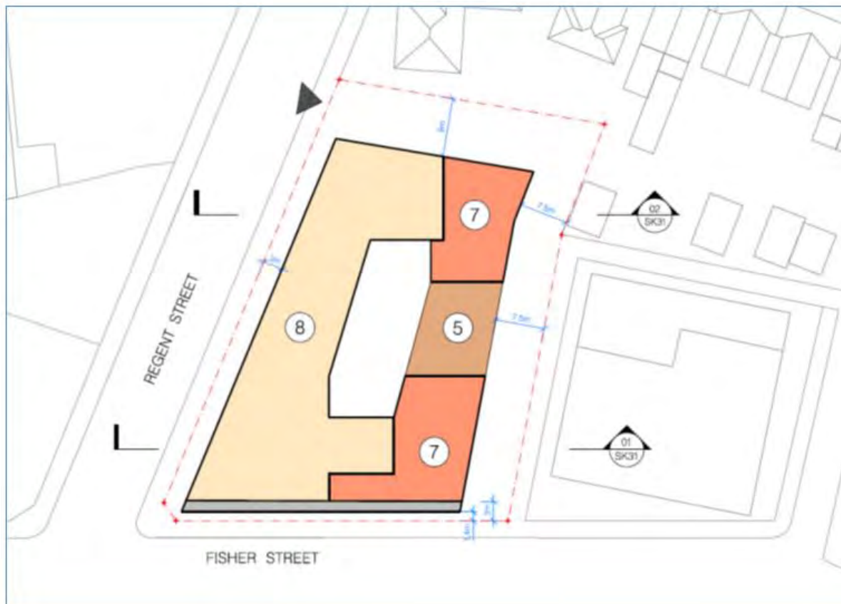
Image 3: Amended building envelope for Site 1 (3-7 Regent Street)
