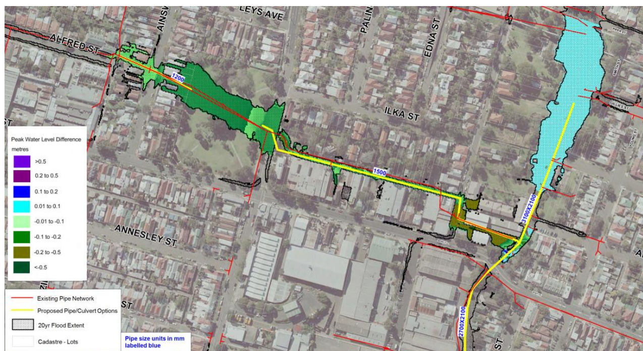
Figure 6-4 Layout of Moore Lane flow path stormwater upgrades [source: Cardno, 2017]
