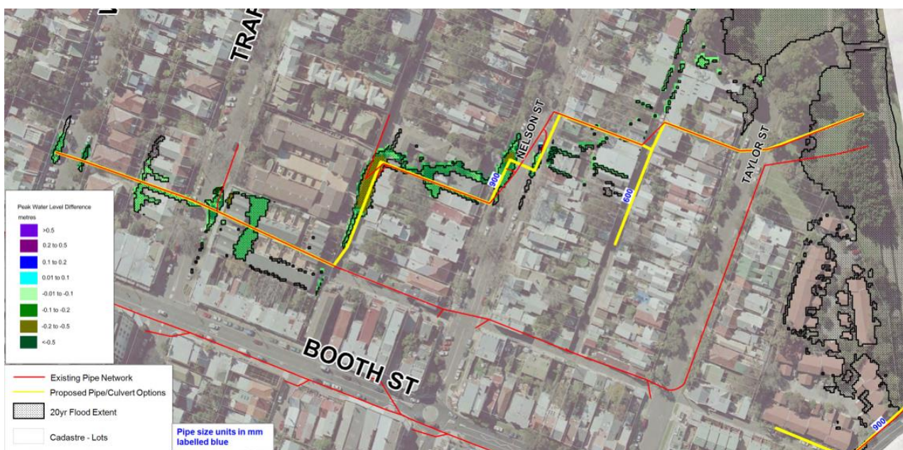
Figure 6-5 Layout of Arthur Street drainage upgrades [source: Cardno, 2017]
